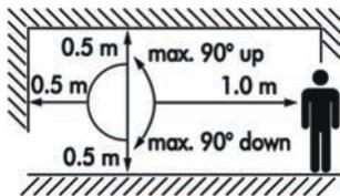
Always observe the minimum distances to persons and flammable objects given on the type plate. Always observe the maximum tilt angle.
